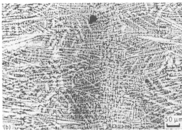
Figure 2 Morphology of austenite in different regions of an EB weldment: (a) columnar morphology at the outer part of the weld pool and (b) equiaxed morphology in the central regions.
